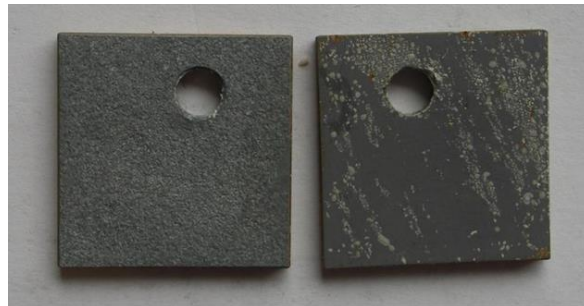
Thermal sprayed Zn samples, front and back after testing.
