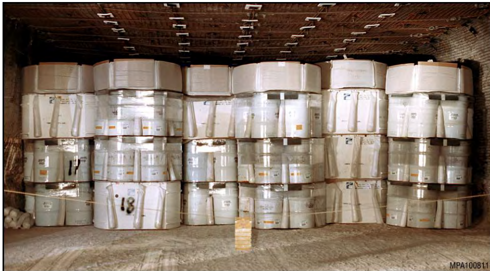
FIGURE 4.1.4-1 Disposal of Contact-Handled Transuranic Waste in Typical 208-L (55-gal) Drum 7-Packs at WIPP (bagged magnesium oxide chemical buffer is on top of each stack) (Source: DOE 2007)
