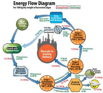
and co-products; developed a continuous flow, two-stage HTL process to separate carbohydrates from the oil fraction—partner Reliance Industries has established the first fully integrated algal biofuels system at Gagwa, India; and carried out extensive LCA/TEA modeling to identify process bottle necks and constraints.
