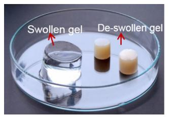
mization of nutrient inputs. We have also developed and tested novel "smart hydrogel"-based solid-liquid separations that allow for low-energy harvesting and effective water recycle without chemical contamination.
