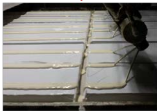
Foam application on manufacturing line
