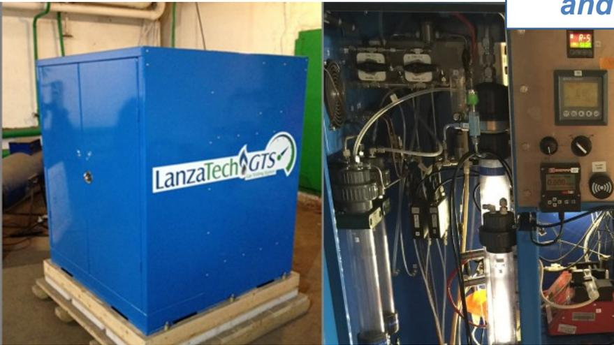
*Continuous operation of mobile fermentation unit integrated with InEnTec pilot gasifier in Richland, WA*
