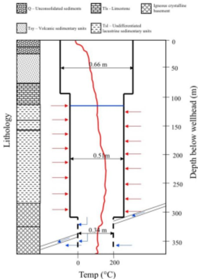
Borehole warming following cold water injection
