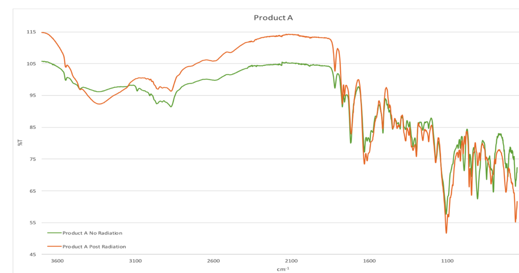
FTIR of irradiated adsorbent illustrating minimal change in the spectra suggesting no change in the adsorbent
