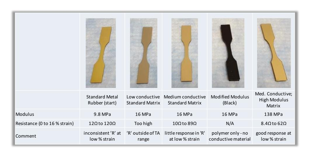
A matrix of Metal Rubber sensor materials were evaluated for modulus and electrical conductivity, based on polymer molecular weight, crosslinking and gold nanoparticle volume percentage.
