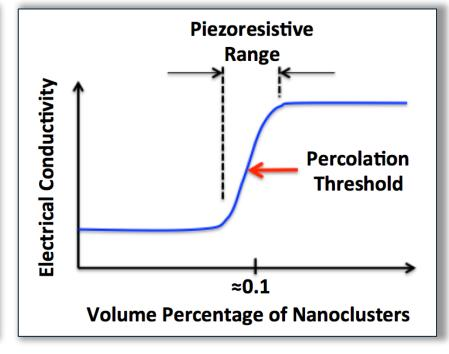
Metal Rubber Sensor performance is controlled via molecular-level properties Percolation Modulus of polymer Type / size of nanoclusters Volume % of conductive nanoclusters
