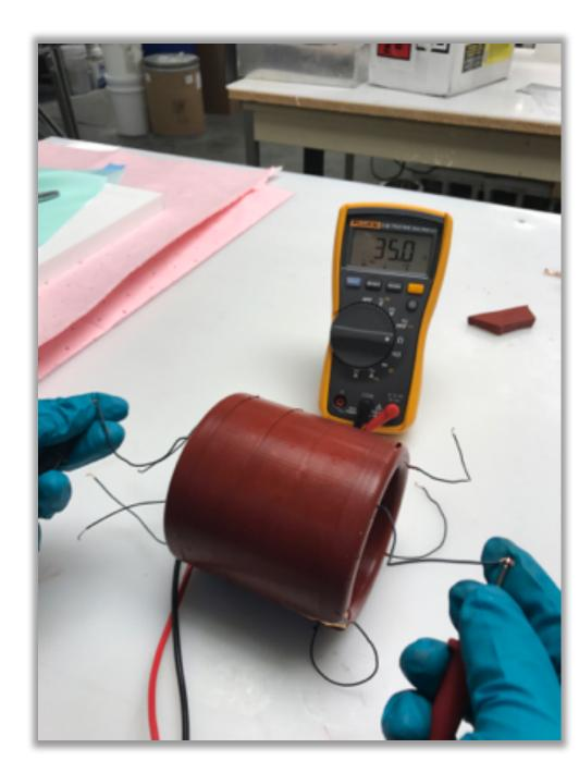
Metal Rubber sensors were evaluated for material compatibility in a high-temperature molding compound used as a packer prototype material. Resistance values before and after sensor integration were similar; approximately 35 Ohms.
