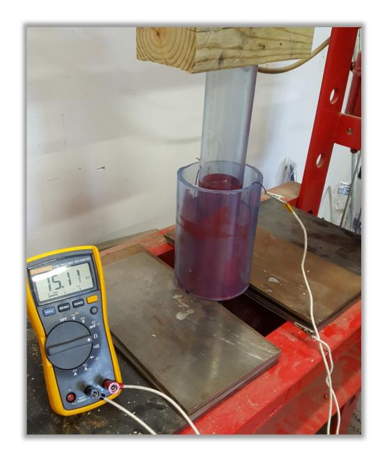
Packer prototype with embedded sensors connected to a multimeter were subjected to initial compression tests using an hydraulic press to approximate stress. Packer prototypes are currently being measured for mechanical stress in tandem with change in sensor conductivity.
