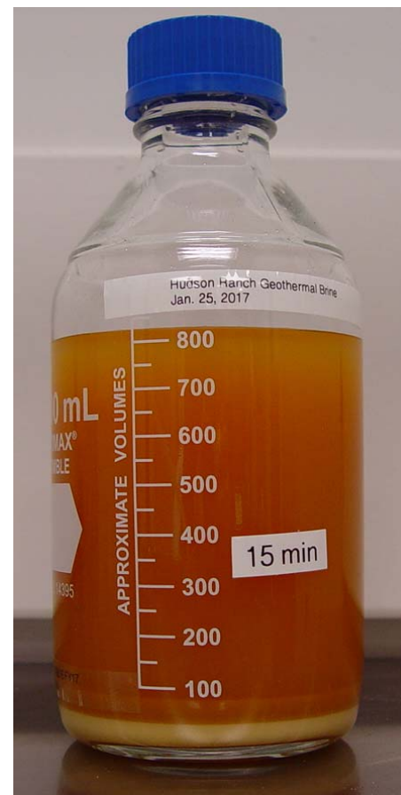
Brine sample taken from well head at Salton Sea geothermal project
