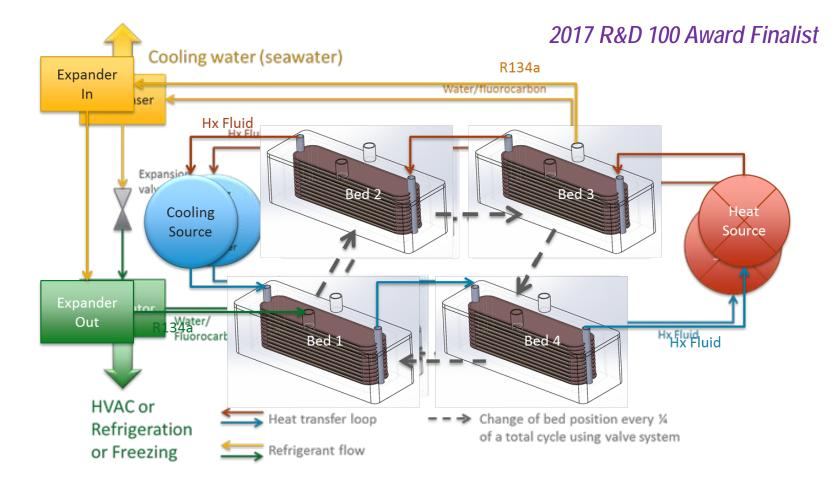
Same thermal compressor system design for cooling can be used to produce power
