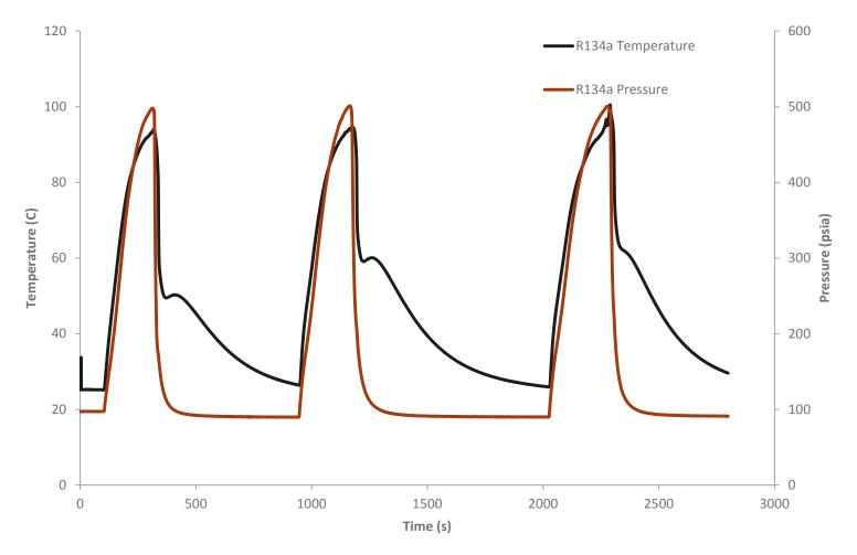
Cycles demonstrate the power of adsorption compression – over 20X more pressure than heating without sorbent
