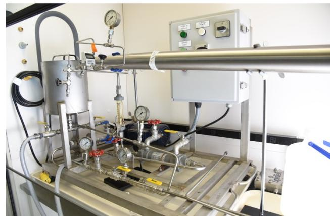
A double staged system with DOW Filmtec NF90 and TW30 membranes is the proposed configuration
