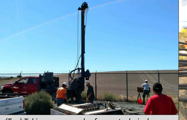
(Top) Taking core samples for geotechnical survey. (Right) Fence dismantled prior to relocation.
