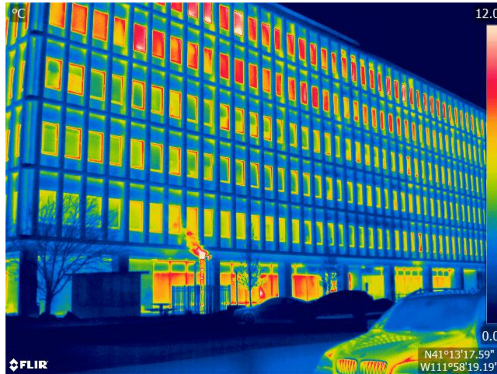
Winter exterior glass surface temperatures, upper floors single clear, lower floors single low-e
