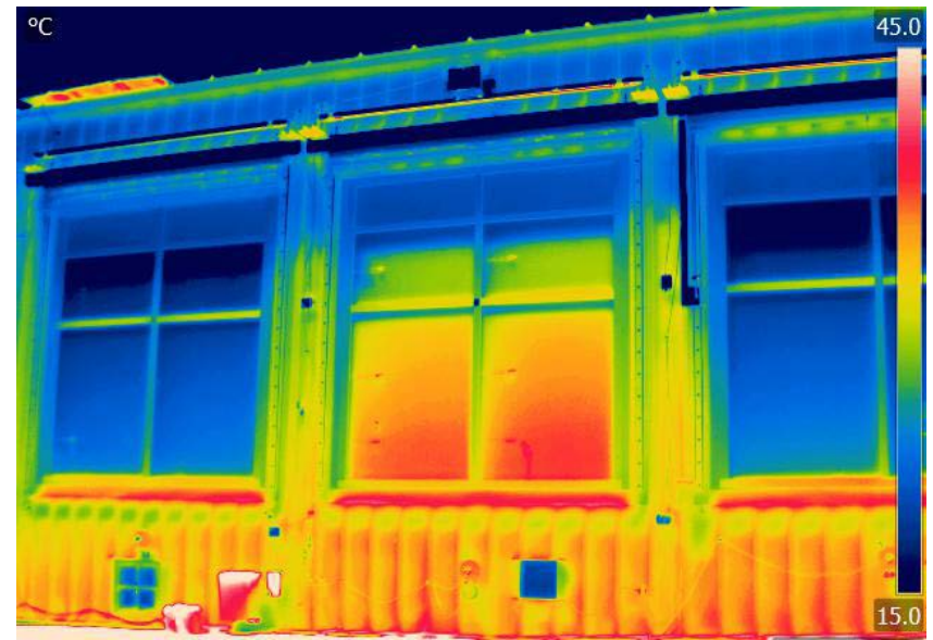
Absorbing glass (center) shown warmer than adjacent windows with uniform background
