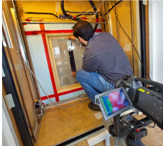
Vertical centerline mirror for collecting specular reflection from enclosure, point by point
