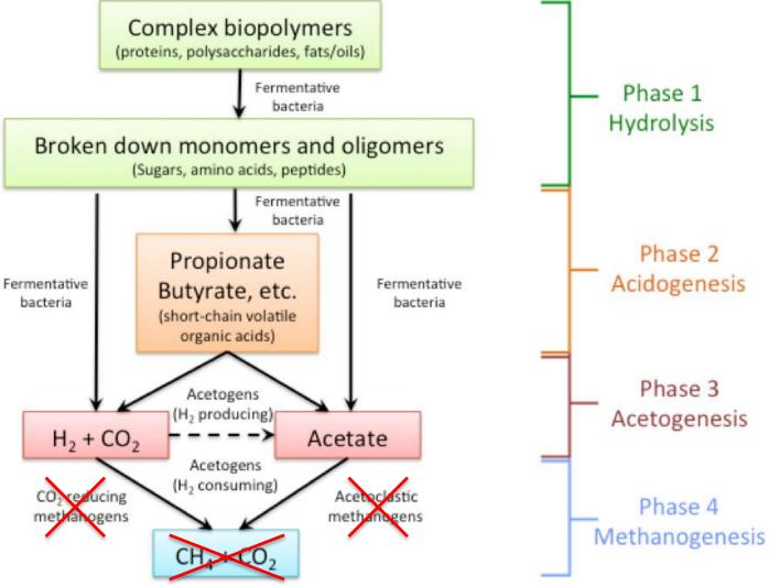
We have developed a novel but simple and low-cost process to convert bio-degradable materials into high value carboxylic acids
