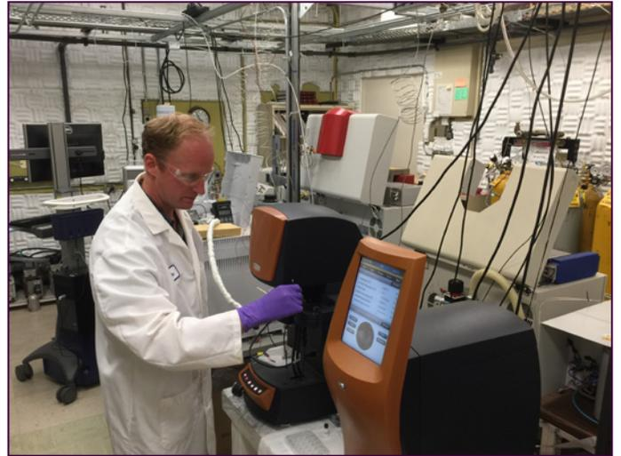
Dr. Michael Singleton of LLNL loads a uranium sample into a thermal gravimetric analyzer attached to an isotope ratio mass spectrometer
