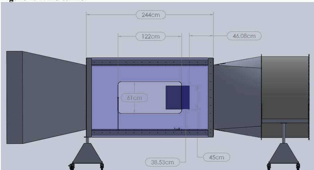
Figure 2. Wind tunnel dimensions
