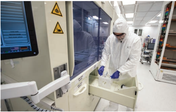
An NREL engineer loads a wafer carrier into the Singulas tool, an automated wet-process station within the newly completed 20,000 sq. ft. (1,858 sq. meters) cleanroom located in the Science and Technology Facility. The new cleanroom and tool will enable reproducible processing of high-efficiency solar cells and collaboration with industry partners and other research laboratories. Photo by Dennis Schroeder, NREL 45985
