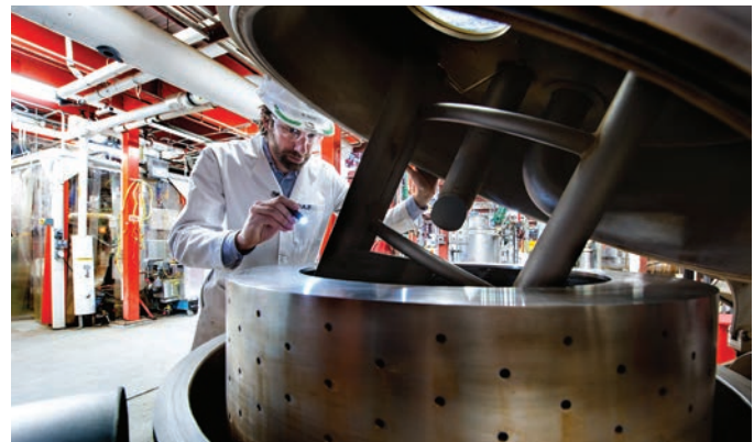
A senior engineer at the Integrated Biorefinery Facility examines a filtering basket centrifuge used in the production of biofuels. Photo by Dennis Schroeder, NREL 35849
