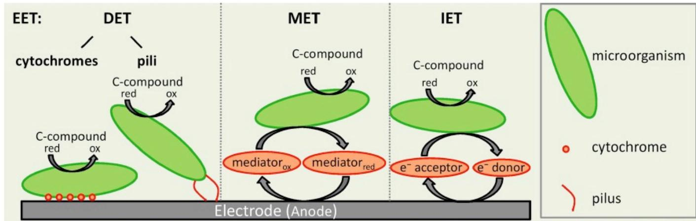
Three possible electron transfer mechanisms
