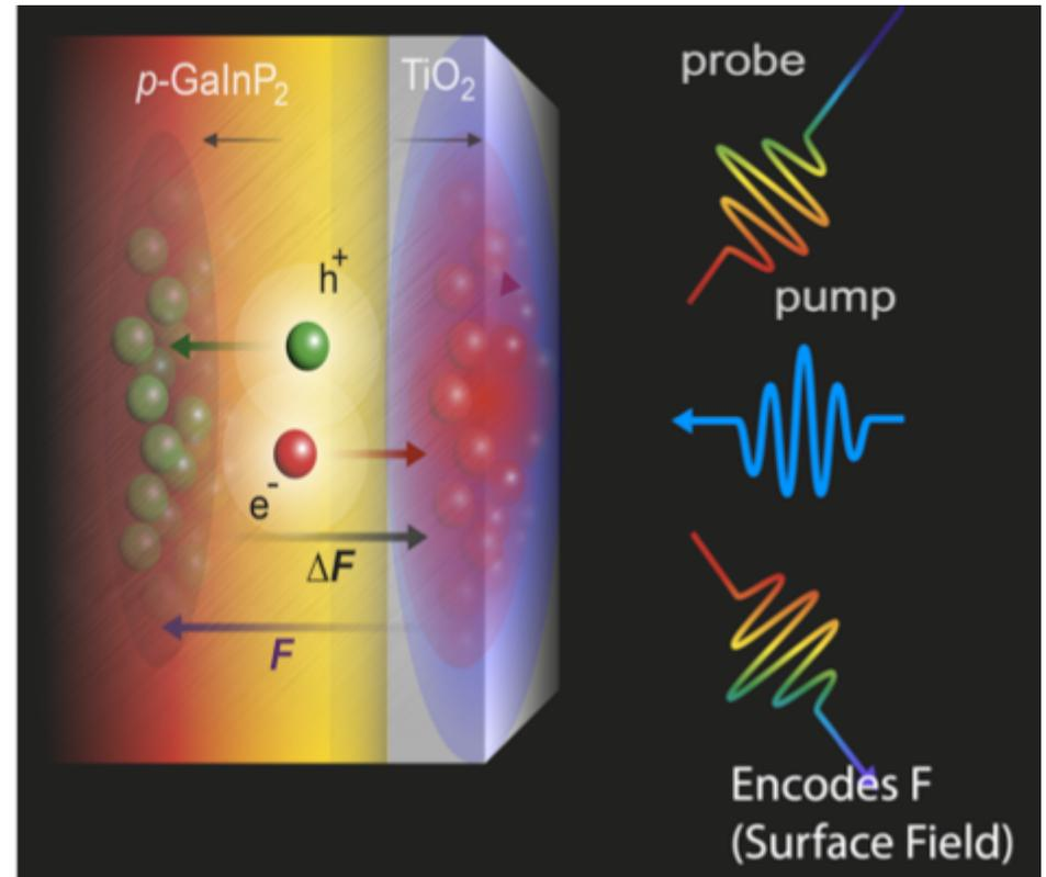
The transient photoreflectance (TPR) technique measures short-lived electrical fields that arise due to charges generated by light that are driven in opposite directions by the properties of the interface.
