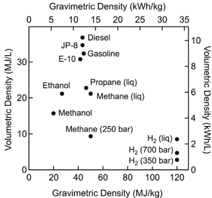
**Figure 1: Comparison of the Volumetric and Gravimetric Densities of Various Fuels**
