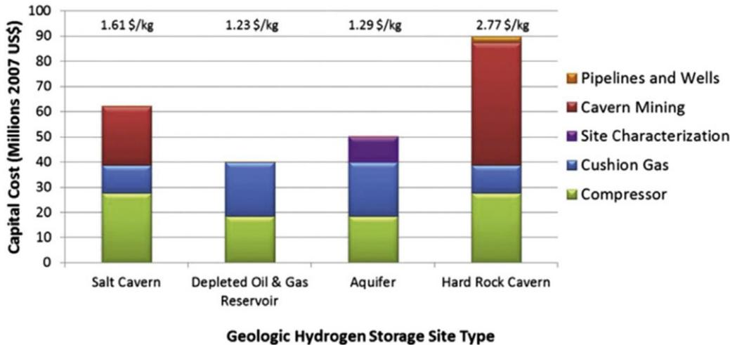
Figure 6. Cost Comparison of Geologic Storage Methods<sup>27</sup>
