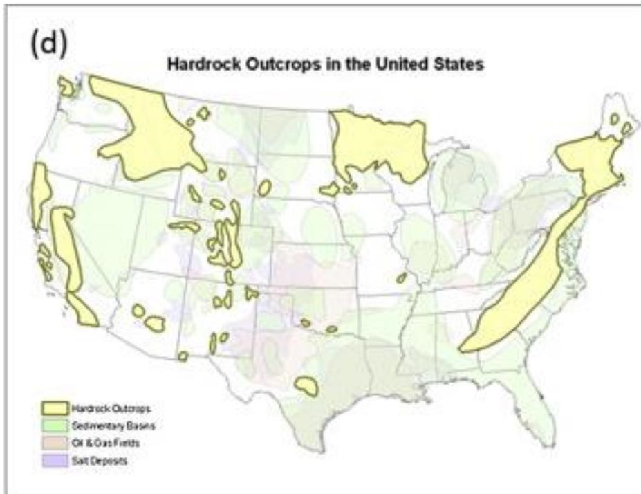
Figure 7. Potential Geologic Storage Sites for Hydrogen in the United States<sup>29</sup>
