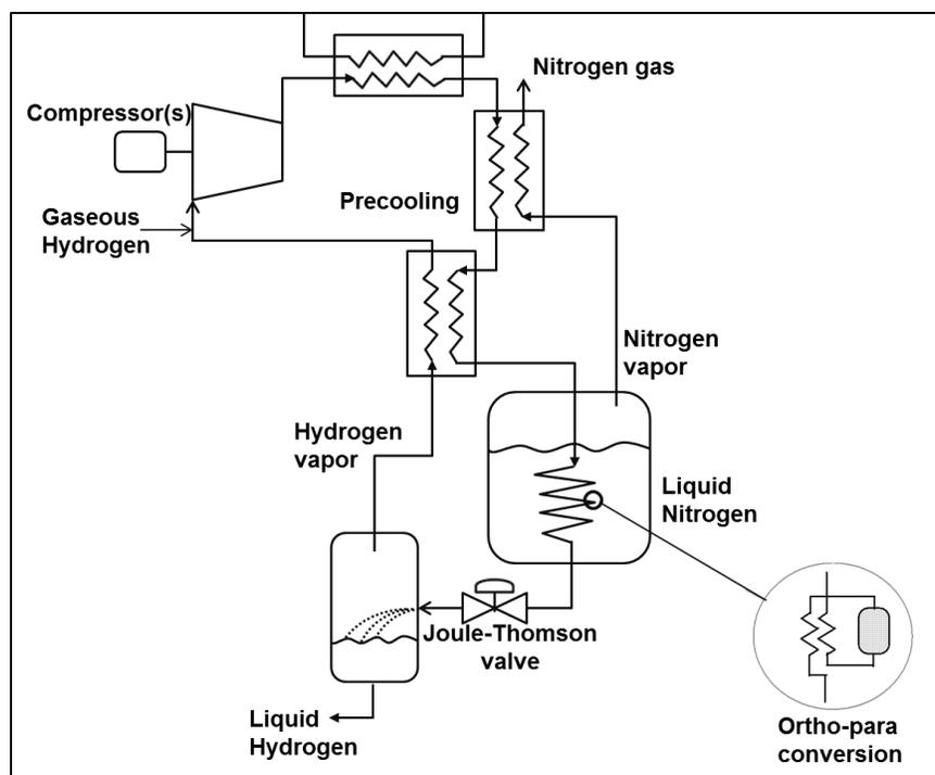
Figure 5. Hydrogen Liquefaction Plant
