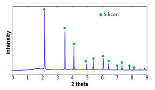
Figure IV-326: X-ray diffraction pattern for µpSi sample tested at ANL confirming the powder composition consists of crystalline Si and small traces of metal oxide
