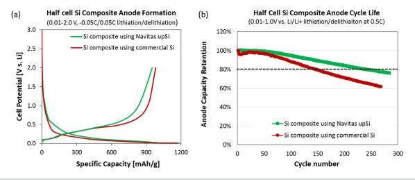
Figure IV-328: Silicon composite made with commercial Si and  $\mu$ pSi (a) half-cell anode formation data (b) cycling performance with 2.0 mAh/cm<sup>2</sup> loading
