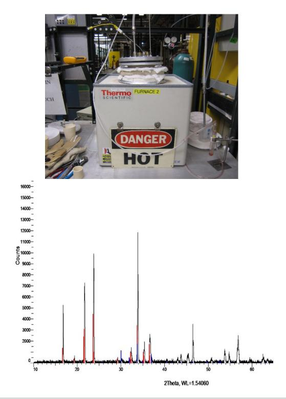
Figure IV-289: (above) Large bore vertical tube furnace for the synthesis of LFO at MERF and (below) overlapped XRD of the original LFO sample and material produced at MERF
