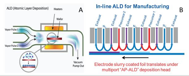
Figure IV-310: (A) Standard "static" or temporal ALD reaction chamber. The coating substrate remains stationary and precursor exposures are separated in time. (B) A conceptual sketch of "spatial" ALD in which a substrate to be coated moves through spatially separated reaction zones
