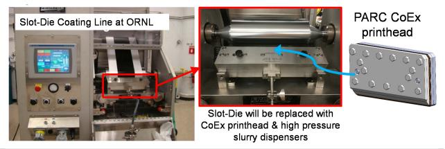
Figure IV-374: Existing electrode coating line at ORNL BMF with planned CoEx integration for this project *Caption Credits/Source (ORNL and PARC)*
