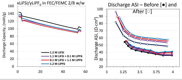
Figure IV-284: Capacity retention vs. cycle number and discharge impedance vs. voltage for NCM523//Si-graphite coin cells
