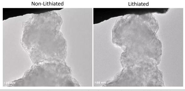
Figure IV-318: TEM observation of down-selected sample 3 (DSS-3) expansion before lithiation (left) and after lithiation (right); the observed expansion was 24% Credits/Source: Chongmin Wang & Langli Luo, PNNL, "Diagnosing failure mechanisms of SI-C nanocomposite anode materials", PowerPoint presentation to Group14 Technologies on 6/16/2016.
