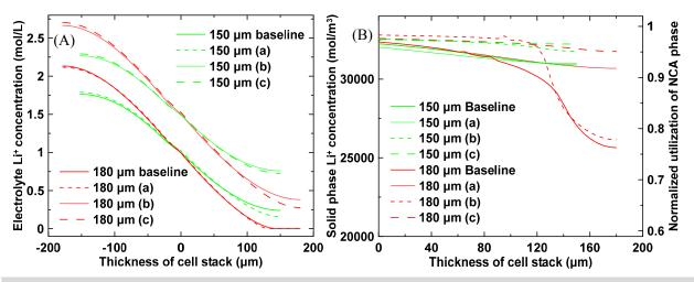
Figure IV-305: The effect of approaches (a) increasing initial molarity, (b) decreasing particle size, and (c) both increasing initial molarity and decreasing particle size on (A) lithium ion molarity profiles in the electrolyte and (B) averaged lithium ion concentration of NCA particles, c\_(s,a), at 1 C discharge upon reaching 2.8 V
