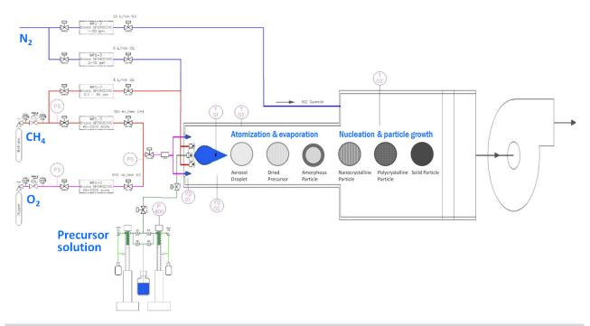
Figure IV-265: P&ID of Flame Spray Pyrolysis
