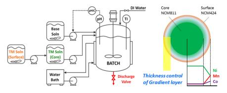
Figure IV-257: 20 L batch reactor and particle structure design for Core-Gradient material
