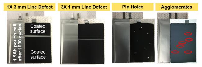
Figure IV-290: NMC 532 cathodes with four different types of defects. Cathodes with each of the different defects were assembled into 1.5 Ah NMC-graphite pouch cells for cycle life testing
