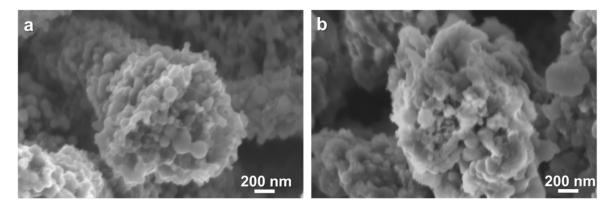
Figure IV-367: Cross-sectional SEM images of Si/C/PAA nanofiber anodes (a) before cycling and (b) after 50 cycles at 0.1 C. The Si/C/PAA weight ratio in the electrodes was 40/25/35.
