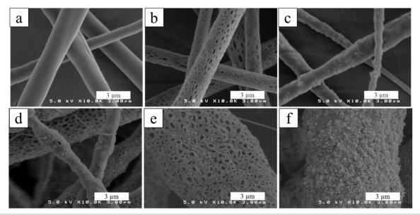
Figure IV-362: SEM images of electrospun (a) PFM/PEO fibers spun at 15% relative humidity, (b) PFM/PEO fibers spun at 75% relative humidity, and (c-f) Si/PFM/PEO fibers containing (c) 20 wt.% Si spun at 15% rh, (d) 35 wt.% Si spun at 75% rh, (e) 50 wt.% Si spun at 75% rh, and (f) 50 wt.% Si spun at 15% rh. The PEO carrier polymer content was 1 wt.% in all samples
