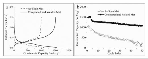
Figure IV-364: Electrochemical characterization of as-spun and compacted/welded Si/C/PAA nanofiber mats: (a) charge/discharge curves and (b) gravimetric capacity over 50 cycles at 0.1 C. The weight ratio of Si/C/PAA was 40/25/35 in both samples
