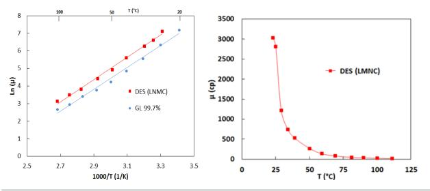
Figure IV-331: Left: Arrhenius plot of the GL and LNMC DES showed a Newtonian fluid behavior of the liquids. 99.7% GL is a product from biomass. Right: The viscosity of the DES precursor for LNMC materials measured within the temperature range
