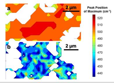
Figure IV-366: Raman maps over an area of ~  $4.5 \times 9.0 \mu m^2$  showing the Raman shift of the maximum peak for Si/C/PAA fiber mat anodes (a) before cycling and (b) after 50 cycles at 0.1 C. White pixels represent regions where the data were omitted due to low spectral intensities (i.e., counts < 10). The electrodes contained Si/C/PAA in a 40/25/35 weight ratio
