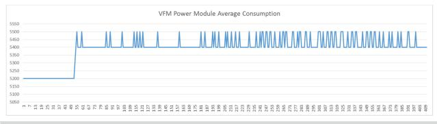
Figure IV-360: Average power consumed by the VFM power module = 5.422 kVA, while the average power consumed by the hot air in process module = 367 VA during a 500 mm/min drying run. Total = 5.422 + 0.367 = 5.789 kVA
