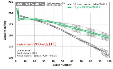
Figure IV-256: Coin cell result of 5  $\mu m$  core NCM811 and commercial NCM811 at 1 C
