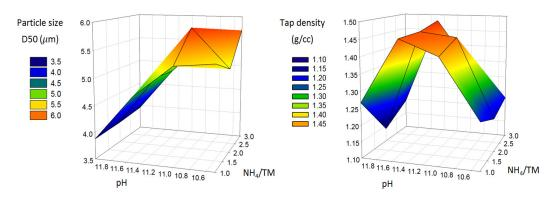
Figure IV-253: 3D mesh plots of precursor particle size and tap density according to pH and ammonium hydroxide ratio to transition metal
