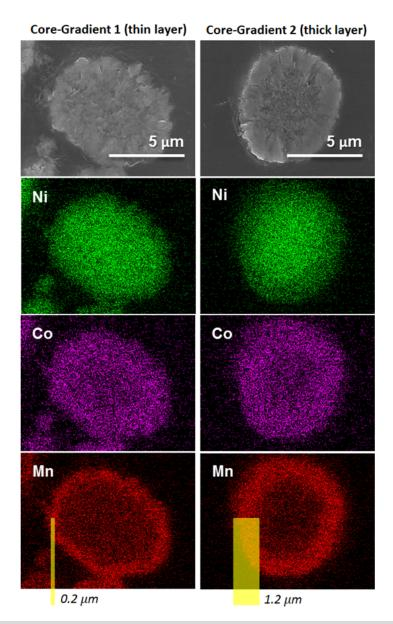
Figure IV-258: Cross-sectional SEM images and elemental mapping of two Core-Gradient materials
