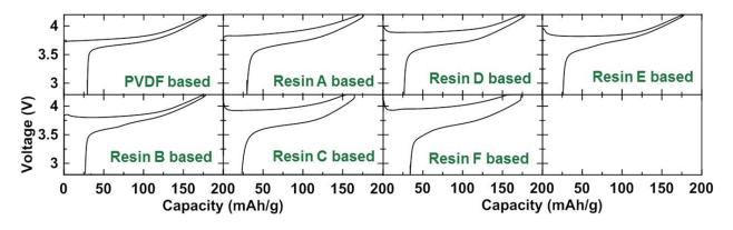
Figure IV-297: Voltage curves of NMC532 composite electrode using different binder system in Li half cells
