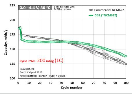
Figure IV-261: 1 C cycling comparison of Core-Gradient 1 and commercial NCM622
