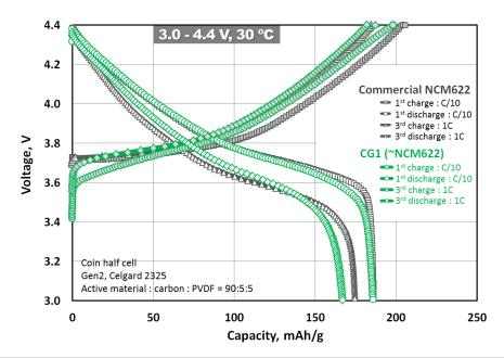
Figure IV-260: Voltage profiles of Core-Gradient 1 and commercial NCM622
