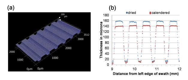
Figure IV-376: CoEx cathode structures. (a) shows the CoEx 1 dried sample print. (b) shows a profile measurement of the dried CoEx 1 print before and after ~12% calendaring. These samples are currently being investigated for electrochemical integrity *Caption Credits/Source (PARC)*
