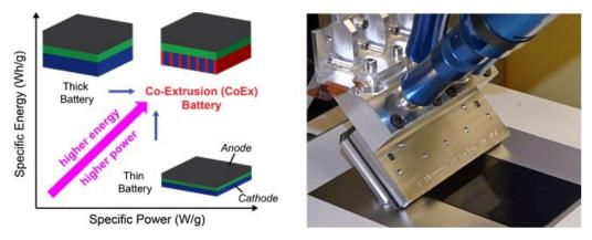
Figure IV-372: (Left) The trade-off space between traditional thick and thin battery electrodes. CoEx can help mitigate the power deficiencies often experiences with thick battery electrodes. (Right) PARC's prototype CoEx battery printhead design for a previous ARPA-E project (DE- DE-AR0000324) Caption Credits/Source (PARC)
