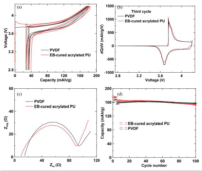
Figure IV-298: (a) Voltage profiles of NMC electrodes using PVDF and EB-cured acrylated PU as binders in Li half-cells; (b) Differential capacity curves of the third cycle for electrodes using different binders; (c) Electrochemical impedance spectra after 3 charge/discharge cycles for electrodes using different binders; (d) Cycling performance of NMC electrodes using PVDF and EB-cured acrylated PU as binders in full coin cells at C/3.
