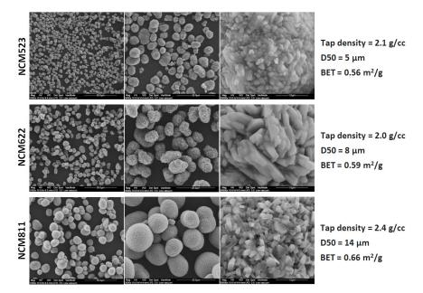
Figure IV-270: NCM materials prepared using 1 L TVR
