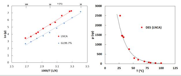
Figure IV-333: Left: Arrhenius plot of the GL and LNCA DES showed a Newtonian fluid behavior of the liquids. 99.7% GL is a product from biomass. Right: The viscosity of the DES precursor for LNCA materials measured within the temperature range
