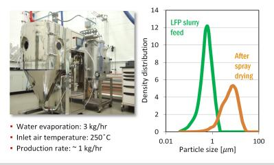
Figure IV-272: Spray dryer and particle size distribution of nano-sized feed and micronized product
