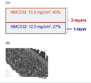
Figure IV-308: (A) illustration of the first design of graded cathode and (B) cross-section image of the electrode
