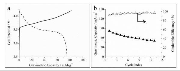
Figure IV-368: Electrochemical characterization of a full cell containing an electrospun Si/C/PAA anode and LiCoO<sub>2</sub>/C/PVDF cathode. (a) Charge/discharge curve collected at 0.1C and (b) Cycling stability over 13 cycles at 0.1 C
