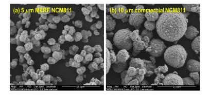
Figure IV-254: (a) Optimized core NCM811 and (b) commercial NCM811 product
