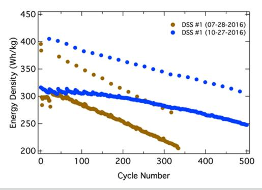
Figure IV-320: Example of gravimetric capacity (Wh/kg) for down-selected sample 1 ("DSS-1") presented on 7-28-2016 compared to the data presented on 10-27-2016
