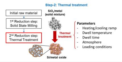
Figure IV-323: Schematic diagram of the 2<sup>nd</sup> step-thermal reduction. Ball milled SiO<sub>2</sub> /metal composite is thermally treated under inert atmosphere and converted to Si/metal oxide. The magnified particle scheme indicates the desirable microstructure for porous silicon formation, where orange is the reduced silicon
