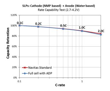
Figure IV-354: Rate capability plots for cells with electrodes dried using conventional and ADP drying methods. All cells were charged at 0.1 C, and discharged at 0.1, 0.2, 0.5, 1.0 and 2.0 C
