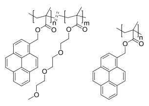
Figure IV-279: Structure of LBNL-PPyE and LBNL-PPy, respectively
