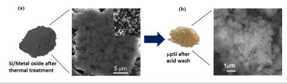
Figure IV-324: SEM micrographs for (a) Si-metal oxide composite structure after thermal treatment, inset shows the microstructures of the metal–SiO<sub>2</sub>; (b) final microporous Si structure
