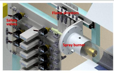
Figure IV-267: Detailed configuration of spray burner system
