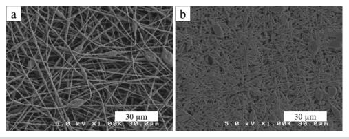
Figure IV-363: SEM images of electrospun mats containing Si nanoparticles, carbon black, and poly(acrylic acid) (Si/C/PAA) in a 40/25/35 weight ratio. (a) an as-spun fiber mat and (b) a compacted/welded fiber mat
