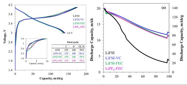
Figure IV-282: Capacity vs. voltage and capacity vs. cycle number for NCM523//Si-graphite pouch cells
