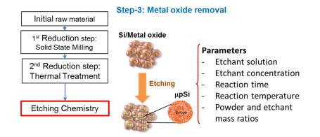
Figure IV-325: Schematic diagram of the metal oxide removal process. The Si/metal oxide is treated using acidic solution to remove the oxide leaving a porous structure
