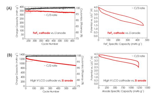
Figure IV-338: Performance of electrochemical cells with conversion-type electrodes: (A) cycle stability and a typical chargedischarge profile of iron fluoride-based cathode cycled against Li anode (capacity is normalized by the mass of the metal fluoride only); (B) cycle stability and a typical charge-discharge profile of Si-based anode cycled against high voltage LCO in matched full cell (capacity is normalized by the mass of the Si-containing composite anode powder)
