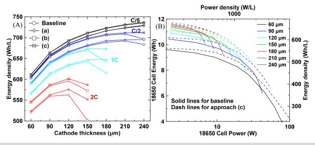
Figure IV-306: (A) the effect of approaches (a), (b) and (c) on (a) average discharge voltages of cell stacks and (b) energy density of cell stacks; (B) The effect of both increasing initial molarity and decreasing particle size on the energy-power Ragone plot of 18650 cells
