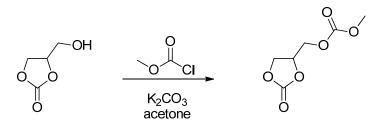
Figure IV-278: Synthesis scheme for GCMC
