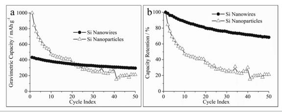
Figure IV-371: Electrochemical performance of as-spun Si/C/PAA nanofiber mats where the Si active material is either in the form of nanoparticles or nanowires: (a) gravimetric capacity and (b) capacity retention over 50 cycles at 0.1 C. The weight ratio of Si/C/PAA was 40/25/35 in both samples
