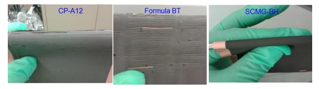
Figure IV-307: Negative electrode flexibility test where electrodes were bent over a 5 mm diameter cylindrical mandrel
