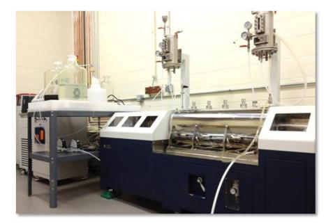
Figure IV-262: Installed 10 L Taylor Vortex Reactor
