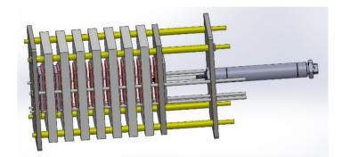
Figure IV-349: Amprius designed a fixture capable of prelithiating eight silicon nanowire anode-based cells "in stack"
