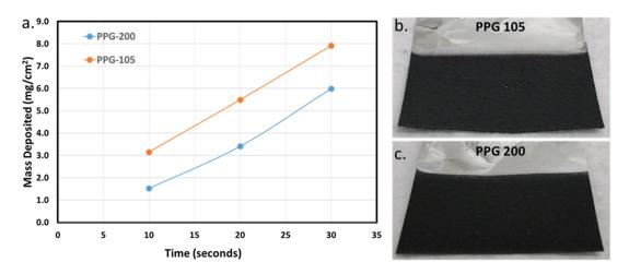
Figure IV-379: (a.) Mass deposited over time for the e-coat formulations using the PPG active material and e-coat binders emphasizing the improved deposition kinetics of the PPG binder system. Photographs of (b) and (c) characterize the film quality and uniformity of the e-coat materials after 20 s of deposition on Al foil
