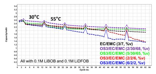
Figure IV-343: Comparison of LNMO full cell performance with control carbonate electrolyte and OS3 containing electrolytes (all with 1M LiPF<sub>6</sub>). Cells are cycled at C/10 for 2 formation cycles and at C/2 for 10 cycles at 30 °C, then continued 50 cycles at C/2 between 3.5 and 4.9 V at 55 °C
