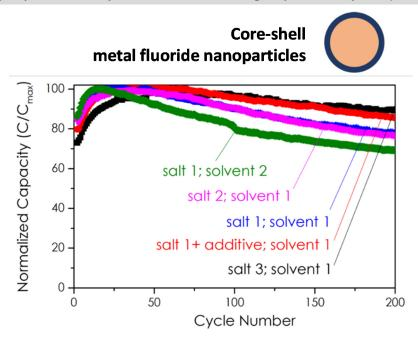
Figure IV-339: Impact of electrolyte composition on electrochemical stability of metal fluoride-based cathode cycled against Li anode
