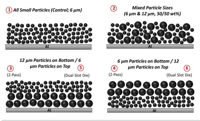
Figure IV-294: Six of the different electrode coatings that are being used to develop the in-line porosity model
