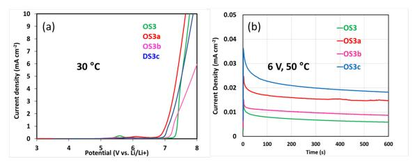
Figure IV-342: a. Oxidative stability comparison at 30 °C; b. parasitic current results at 6 V and 50 °C of OS3 family electrolytes
