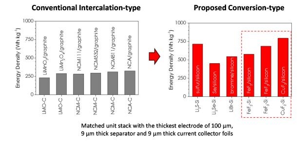
Figure IV-336: Estimation of the specific energy of unit stacks (calculating units) in rechargeable Li batteries achievable with commercial intercalation-type electrodes and selected conversion-type electrodes. Areal capacities of anodes and cathodes were matched 1:1 and no extra capacity was considered for the formation losses
