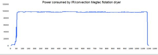
Figure IV-359: The average power consumed by IR/convection dryer during a 500 mm/min drying run = 9.727 kVA
