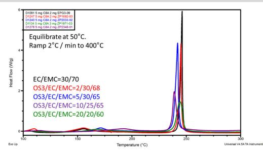
Figure IV-344: Differential scanning calorimetry (DSC) test results for de-lithiated LNMO cathodes formed with various HV electrolyte formulations: Carbonate control (black), 2% OS3 (red), 5% OS3 (blue), 10% OS3 (purple), and 20% OS3 (green)
