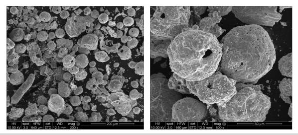
Figure IV-334: The LNMC powders produced in Gen 1.1 reactor
