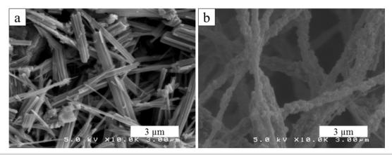
Figure IV-370: SEM images of (a) Si nanowires and (b) electrospun nanofibers containing Si NWs, carbon black, and PAA in a 40/25/35 weight ratio
