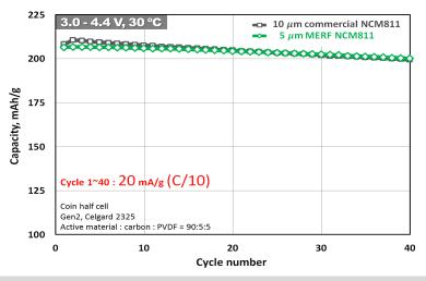
Figure IV-255: Coin cell result of 5  $\mu m$  core NCM811 and commercial NCM811 at C/10
