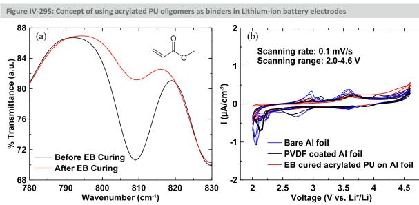
Figure IV-296: (a) FTIR spectroscopy around 810 cm-1 of acrylated PU before and after EB curing; (b) CV of bare Al foil, PVDF coated Al foil and acrylated PU coated Al foils after EB curing
