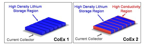
Figure IV-373: Illustrations of proposed CoEx 1 and CoEx 2 structures. CoEx 1 is a corrugated structure with open channels for electrolyte to fill the electrode structure. CoEx 2 is a structure where a more conductive or porous version (red) of the dense blue region will be deposited *Caption Credits/Source (PARC)*
