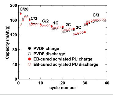
Figure IV-300: Rate performance of NMC composite electrodes using PVDF and EB-cured acrylated PU as binders
