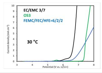
Figure IV-341: Oxidative stability comparison at 30 °C of OS3 vs carbonate control vs fluorinated electrolyte
