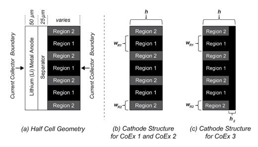
Figure IV-375: Illustrations of the CoEx structures modeled in COMSOL. Region 1 represents a 90/5/5 (NCM523/PCVDF/Carbon Black) Composition with 33.6% porosity while Region 2 represents pure electrolyte for the CoEx 1 and 3 structures and a more porous formulation of the 90/5/5 composition for CoEx 2 *Caption Credits/Source (PARC)*
