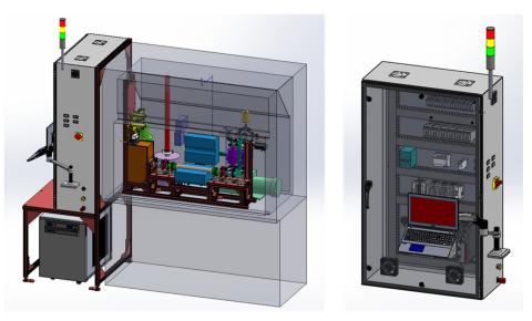
Figure IV-337: Schematic of the designed and assembled tool for use in metal fluoride cathode synthesis: (left) view of the entire system, (right) automation control panel
