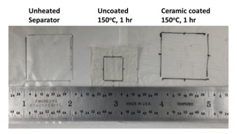
Figure IV-350: UV Ceramic coating affords the separator dimensional stability when heated to dangerous temperatures, like 150oC for 1 hour
