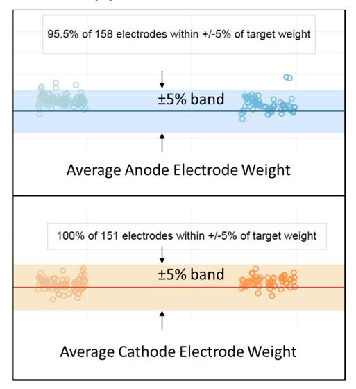
Figure IV-385: Plot of average anode and cathode electrode weights for large-format (> 250 cm<sup>2</sup>) semisolid electrodes produced on 24M's Gen2 prototype line
