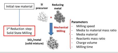
Figure IV-322: Schematic diagram of the 1st step reduction/activation. SiO<sub>2</sub> and reducing metal are mechanically milled to pre-activate the solid system and partially reduce the oxide
