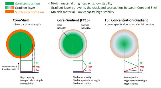
Figure IV-251: Typical particle structure of gradient materials
