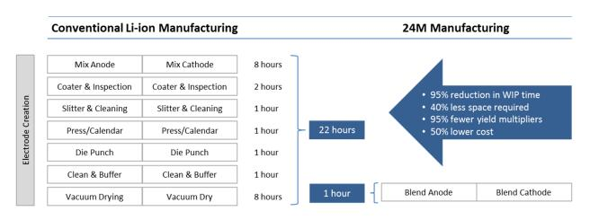
Figure IV-384: Comparison of 24M's novel manufacturing processes to conventional lithium-ion manufacturing approach, highlighting the dramatic reduction of complexity in the electrode creation steps
