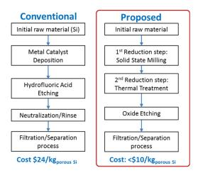
Figure IV-321: Conventional production of porous silicon uses hazardous hydrofluoric (HF) acid and expensive metal catalyst. Navitas route reduces cost and impact, using SiO<sub>2</sub> raw material and no HF
