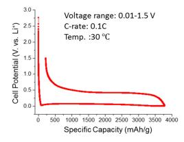
Figure IV-327: Voltage-capacity plots for µpSi electrode formation, with ~3600mAh/g reversible capacity and 7% ICL
