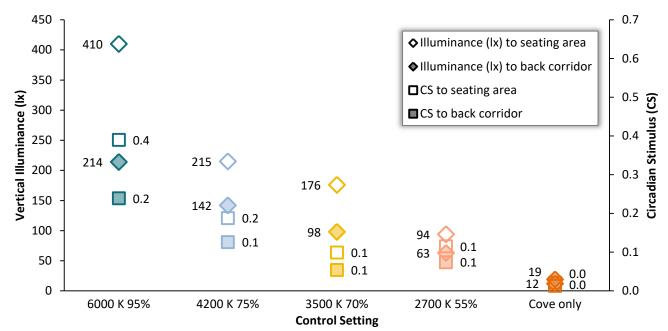
**Figure 10.** Scene Illuminance and CS: Second Measurements, September. The SPDs were measured with the CL-500A at seated eye height for one of the seating locations at a table in the dining/activity area in the direction facing toward the seating area in the dining/activity area and also in the opposing direction toward the back corridor. Measurements were made for each of the five lighting scenes evaluated during the second commissioning.
