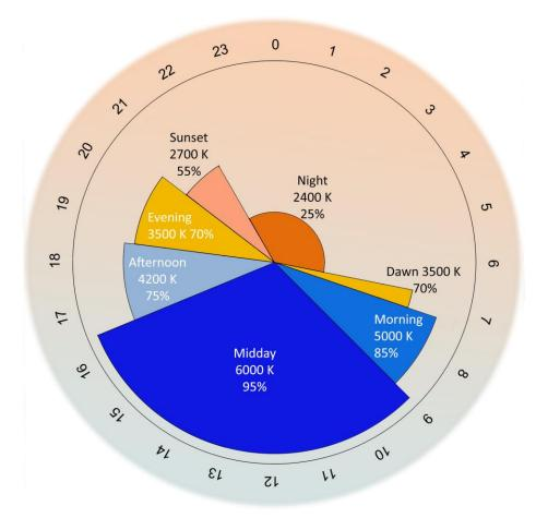
Figure 2. Daily schedule for the SPD and intensity level control setting: initial. The figure shows the initial schedule for the changes in SPD, indicated by CCT, and intensity level control setting throughout the day. The intensity level is expressed as a percentage of full output. The downlights and coves in the dining/activity area and the coves in the corridors initially changed according to this schedule.
