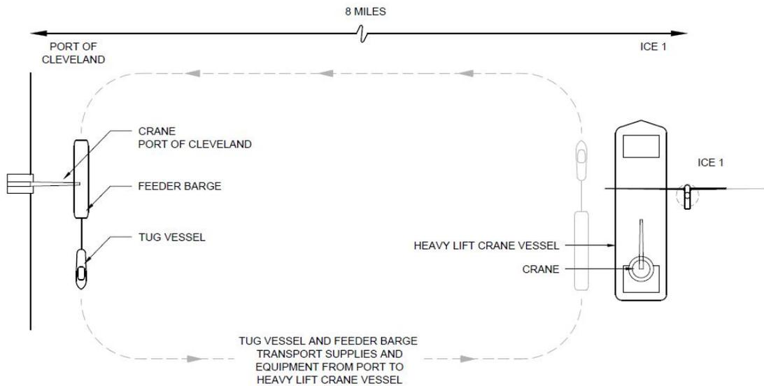
Inset 2. Installation Vessel Plan View
