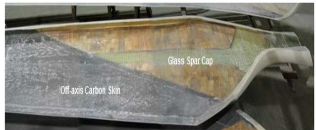
DOE-designed carbon-fiber hybrid blade for passive load
