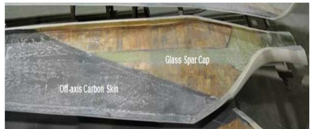
DOE-designed carbon-fiber hybrid blade for passive load
