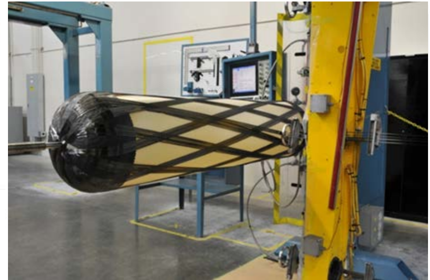
COPV manufacturing process via filament winding (Credit: Quantum Technologies, 2012)
