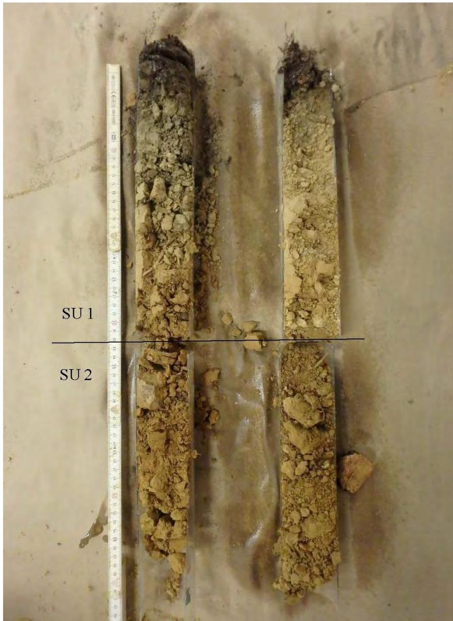
**Figure 3. Core 1 and 2 soil samples, exhibiting the SU 1 and SU 2 profile sequence.**
