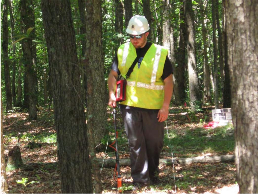
**Figure 2-1. Magnetic susceptibility survey conducted at site 33PK347, view to the north.**
