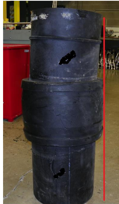
Figure 5: The pipe end and couplings were not properly aligned.
