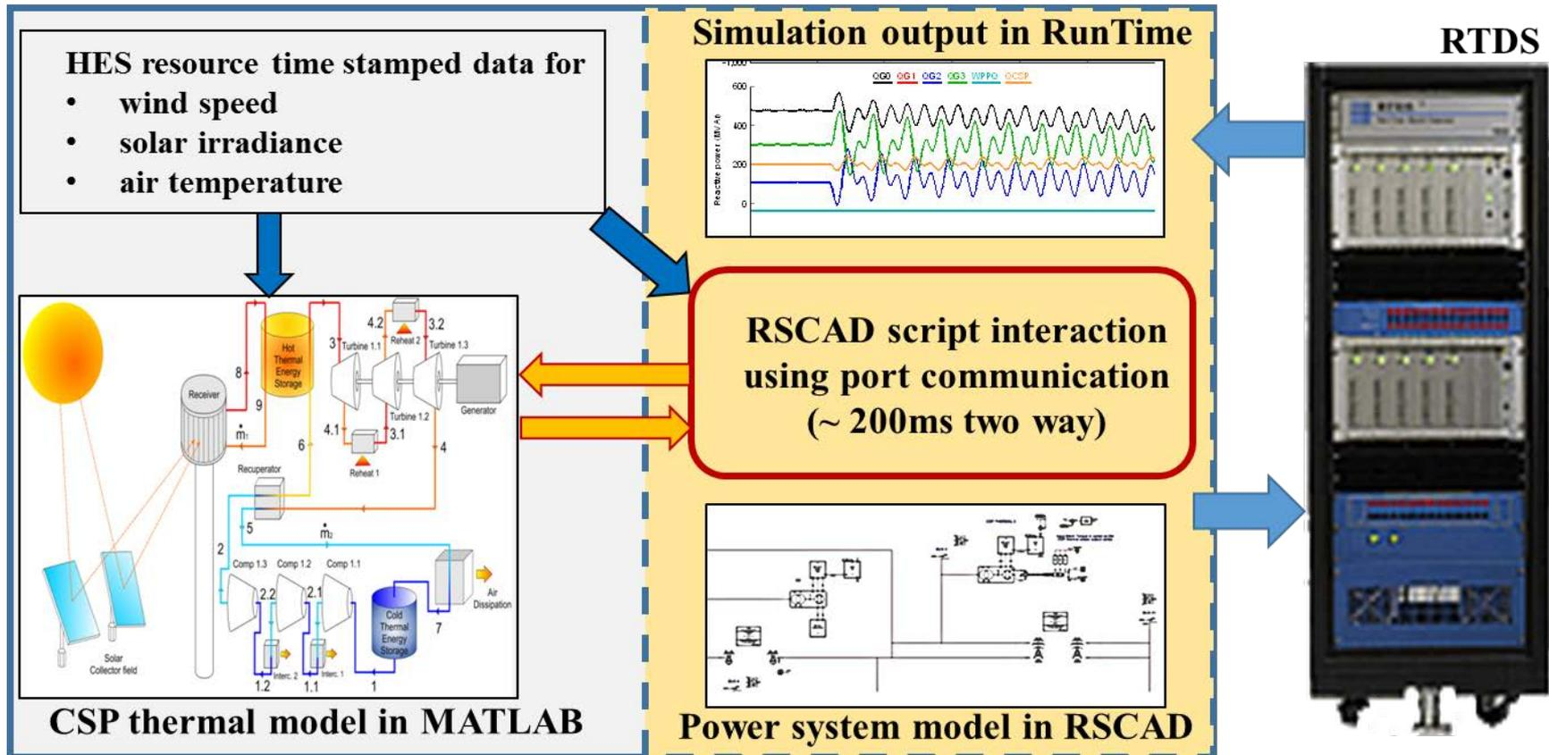
**RT co-simulation of electrical-thermal-mechanical systems with physics based models**
