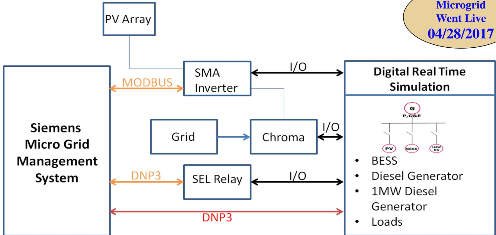
Fig. 5 BLR Microgrid Setup and HIL Testing
