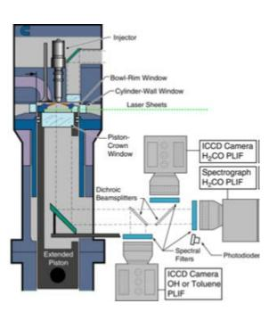
Toluene Fuel Tracer PLIF (Genzale et al. SAE 2009, Kokjohn et al. Comb. Flame 2015)
