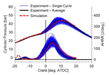
LES using CONVERGE with dynamic structure model and validated reaction mechanism
