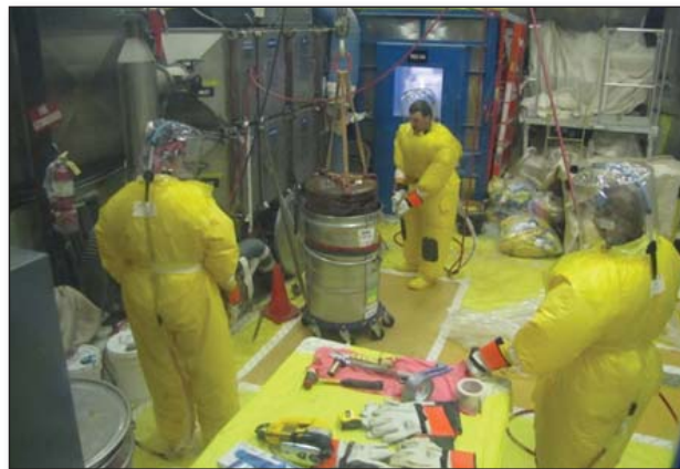
Workers at the TWPC wear protective ‘bubble suits’ while working with contact-handled TRU waste.
