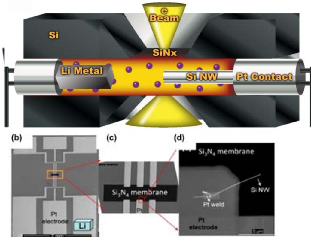
In-situ liquid cell for battery study; a new cell can be designed for electrocatalysts study.
