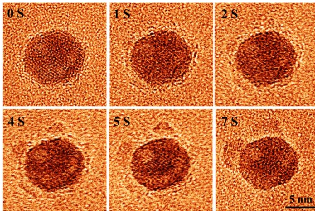
Atomic-scale reaction dynamics of a single Pt<sub>0.5</sub>Co<sub>0.5</sub> nanoparticle in an oxidizing environment (0.1 mbar O<sub>2</sub>, 250 °C)
