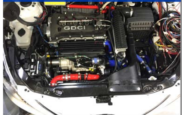
Gen3 mockup engine installed in a test vehicle
