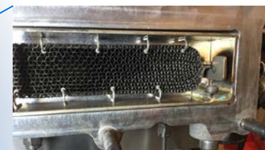
Low mass , fast, electric intake air heaters
