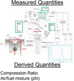
Compression Ratio Air/fuel mixture (phi) T<sub>IVC</sub>, T<sub>EVO</sub>, T<sub>exhaust</sub>, T<sub>residuals</sub>, T<sub>BDC</sub> X<sub>i</sub> (actual) %residual, %EGR %water removal in EGR loop %water removal upstream gas analyzers IMEP, heat release, Ringing Intensity
