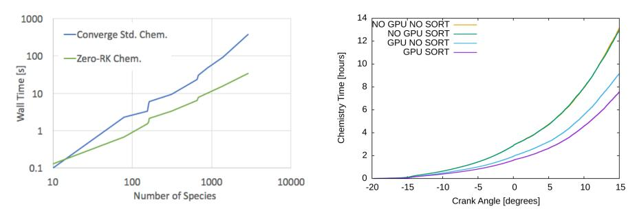
CPU only scaling with comparison to ConvergeCFD built-in chemistry (5.5x faster at 1000 species)
