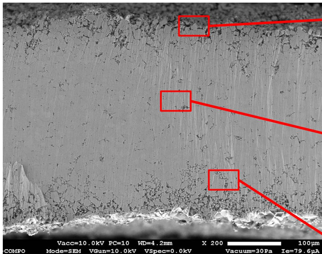
Nearly all grains converted to  $\beta$  throughout thickness of pellet (agrees with XRD findings).
