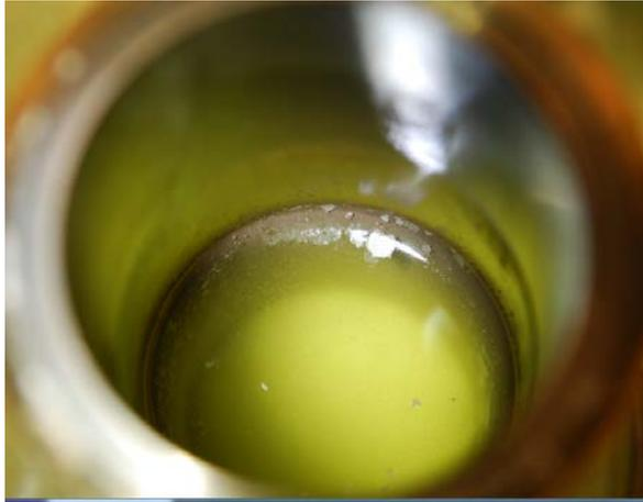
Particulate deposition visible on vessel dip tubes
