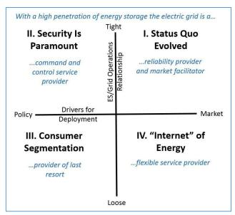
that interfaces with the electric grid. In the loosely integrated scenarios, the electric grid operator does not control dispatch, deployment, and/or design. Under these two impact axes, the Subcommittee developed four distinct and different future scenarios of HPES and resulting grid impacts as indicated in the graphic.
