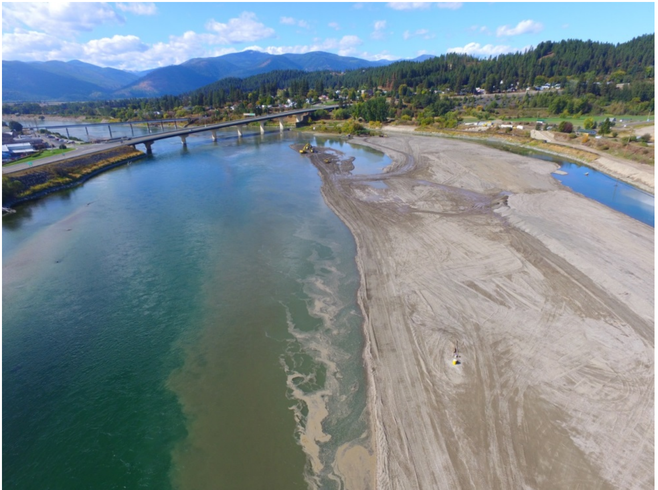
Figure 11. Sediment plume during 2015 Island Construction
