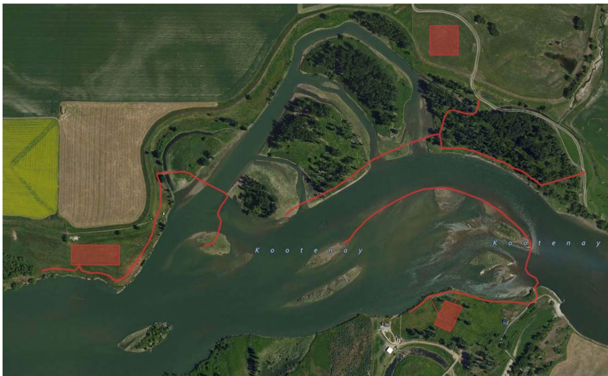
Figure 8. Staging areas and temporary haul roads
