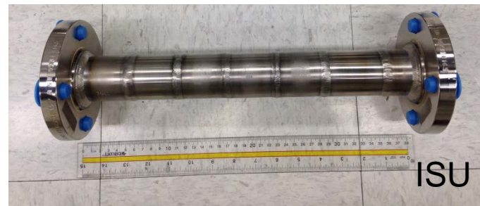
Alloy coupons and spool piece for exposure in biomass liquefaction systems
