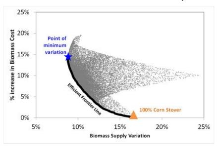
The Efficient Frontier (black curve) indicates Pareto efficient, lowest biomass cost for a given supply risk (variation). The triangle represents 100% corn stover. The star represents the point of the minimum supply variation through diversification of corn stover with switchgrass and wheat straw (approx. at the ratio 2:1:1). The grey area is simulation output (Golecha and Gan, 2016)
