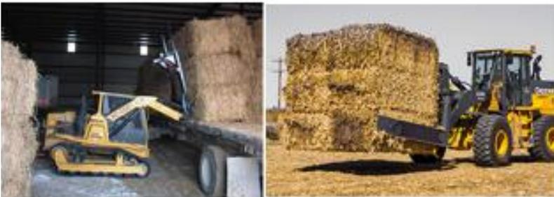
Typical trailer loading / unloading; 1 to 6 bales at a time; 20-40 minutes
