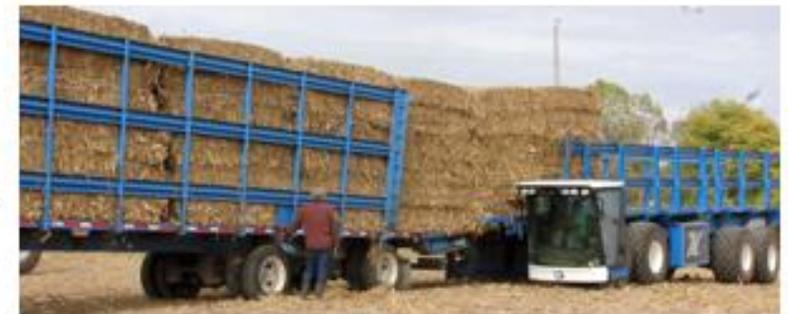
Self-Loading / Unloading trailers; 36 bales at a time; 5-10 minutes
