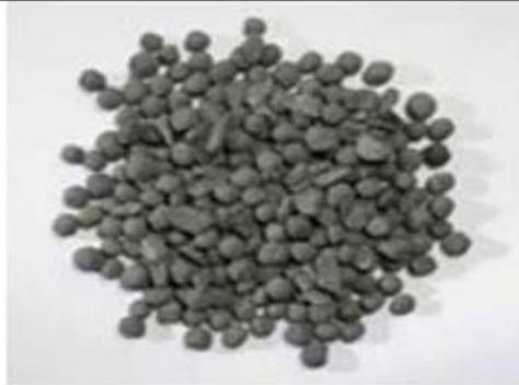
**Direct Reduced Iron:** DRI is typically produced in pellet form and can be loaded directly into an EAF, Blast Furnace, or Basic Oxygen Furnace. It contains a very high iron content (typically >90%). DRI exits the DRI module at a high temperature, and can be fed directly into furnaces as a means to reduce energy costs.
