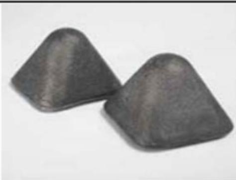
**Merchant Pig Iron:** MPI is produced in a blast furnace and cast into small "pigs" suitable for transportation. MPI has a higher iron content (around 96%) and less slag elements than DRI or HBI, and will typically sell at a premium. That said, MPI, HBI, and DRI are all substitutes for one another.
