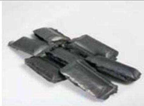
**Hot Briquetted Iron:** HBI is a compressed form of DRI that facilitates easier transportation and handling. HBI is formed as DRI exits the module, and it compressed while still hot. DRI reacts more easily with water and requires tighter standards for shipment; HBI is less reactive and ships easier.
