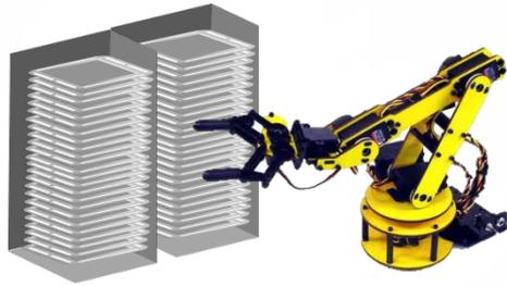
Pick-and-Place robot picks up and orientates anode and cathode BPPs into welding single fixture, then removes after welding. (20 seconds)
