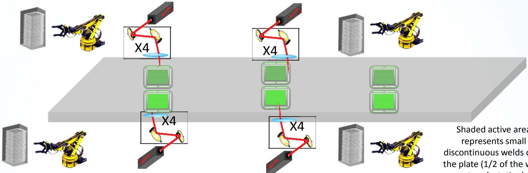
Shaded active area represents small discontinuous welds over the plate (1/2 of the weld at each station)
