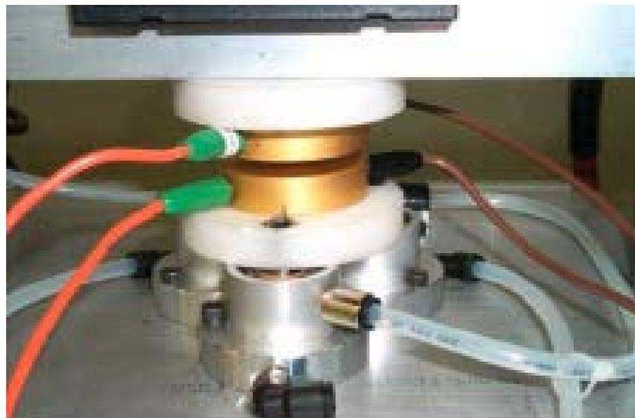
Measured across the bipolar plate; includes interfacial contact resistance (on as received and after potentiostatic test), measured both sides at 200 pounds per square inch ( $138 \text{ N/cm}^2$ ), H. Wang, M. Sweikart, and J. Turner, "Stainless steel as bipolar plate material for polymer electrolyte membrane fuel cells," *Journal of Power Sources* 115 (2003): 243-251.
