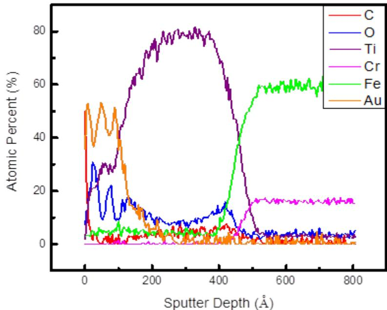
AES depth profile of multi-layer coating structure on the stainless steel substrate (316L), before and after the corrosion tests.
