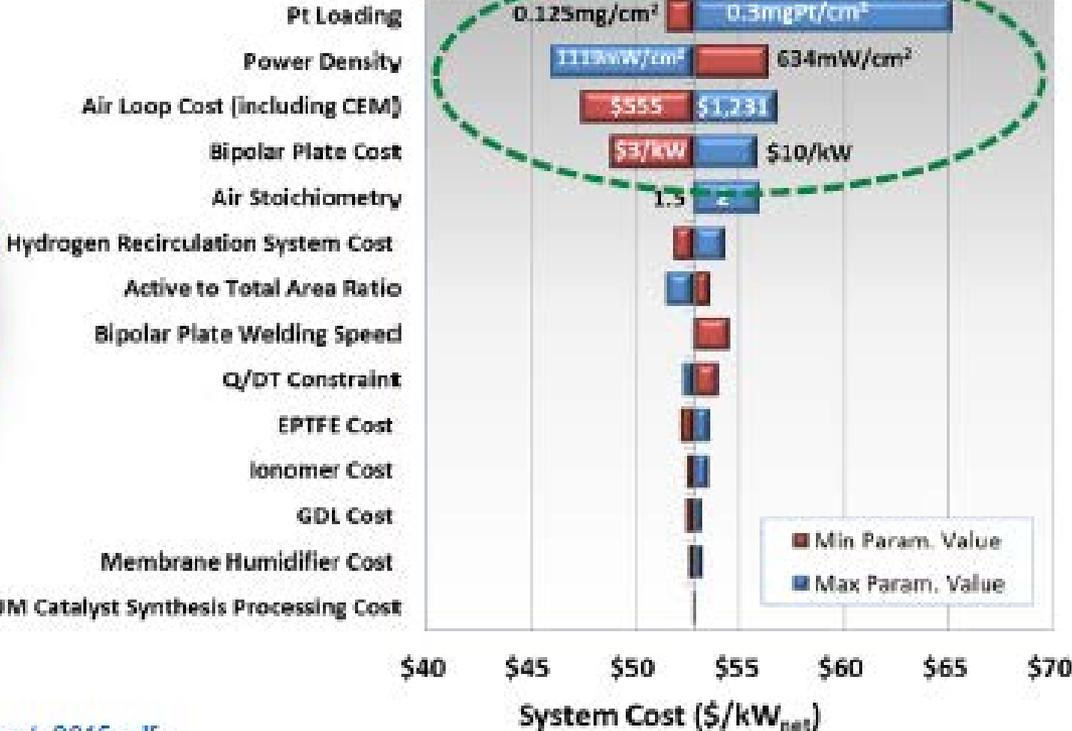
**Bipolar plate is one of the most sensitive cost factors. Cost reduction (materials and manufacturing process) is required.**
