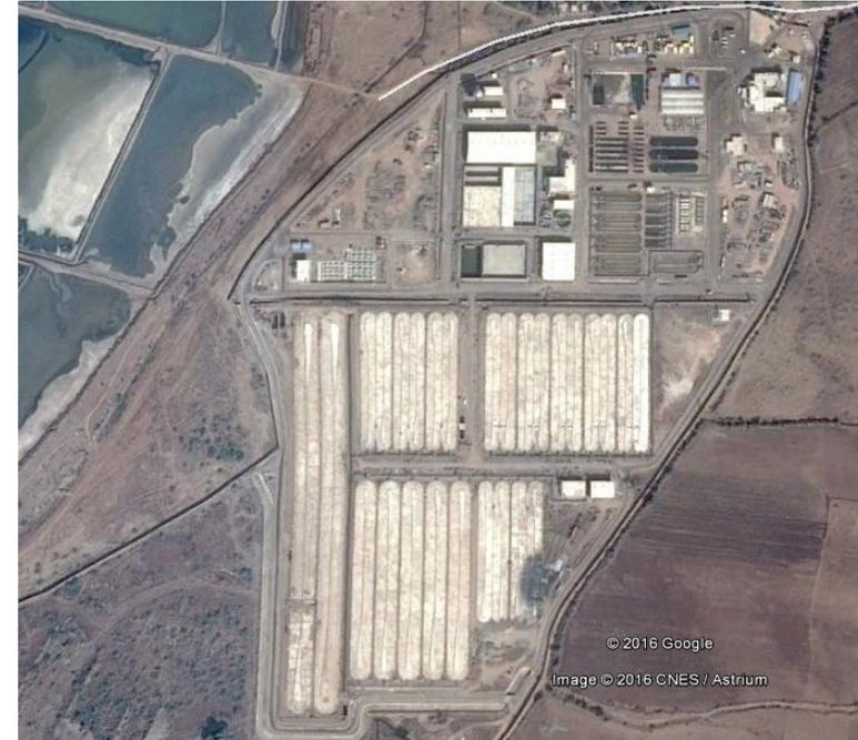
**Image of RIL Gagwa facility.** Longer ponds on left are over 1 km long. Includes harvesting, HTL, media mixing, central control room. Refinery nearby.
