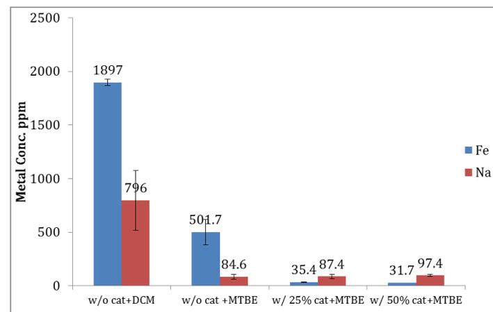
Figure 2. Fe (blue) and Na (red) concentrations (ppm) in biocrude from HTT at 400 °C, 60 min
