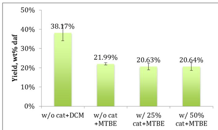
Figure 1. Biocrude yields from HTT at 400 °C for 60 min
