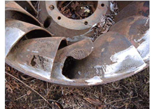
Francis turbine: cavitation damage and old repairs with stainless steel welding.
