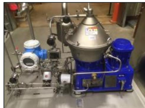
Performance testing of a new disk stack centrifuge is under way.
