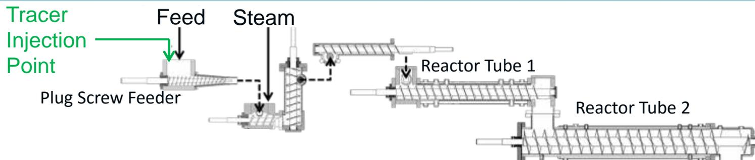
At the last peer review meeting, we reported on the successful development of an on-line technique to measure RTD using a NaCl tracer detected by conductivity.
