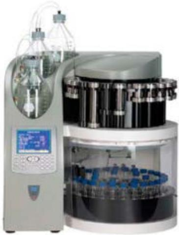
Bench Scale Extraction Reactor (Flow-Through)
