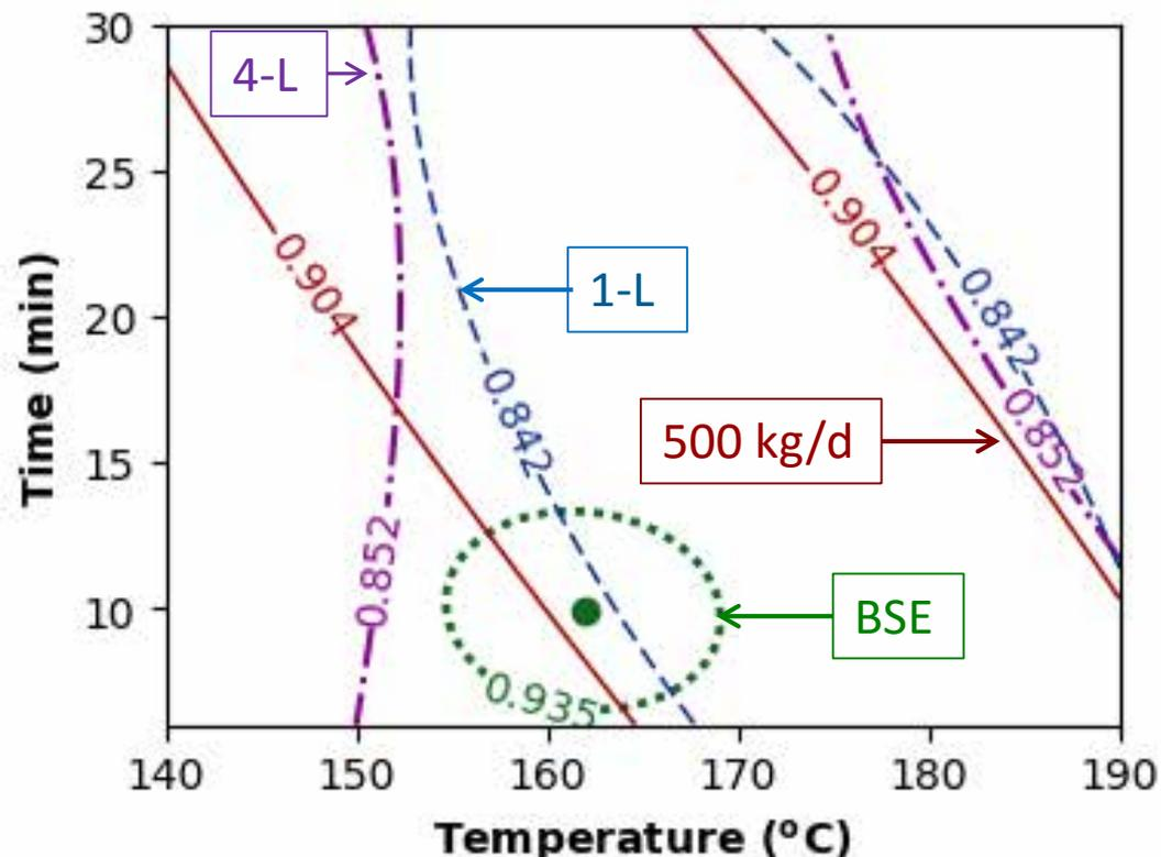
Plot shows the predicted maximum total xylose yield (96%) for the BSE reactor (green point) and yields at two standard deviations from the optimum for all reactor systems.
