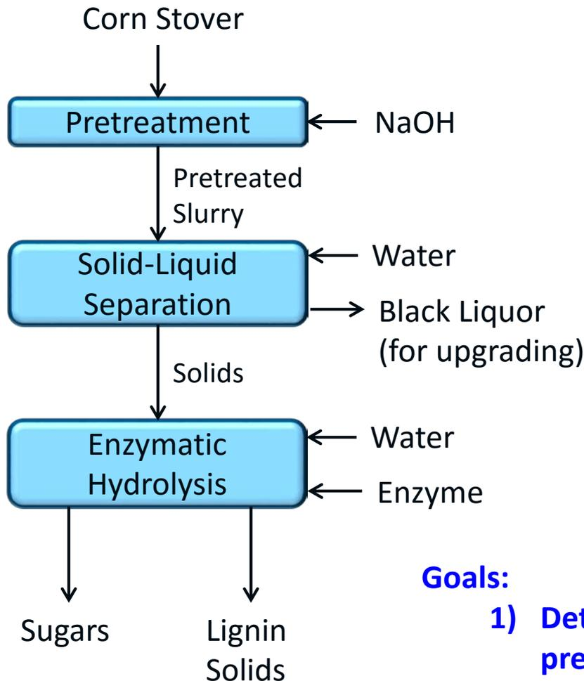
**Pilot-scale alkaline pretreatment was researched as one method of obtaining soluble lignin for valorization (with Lignin Utilization project).**
