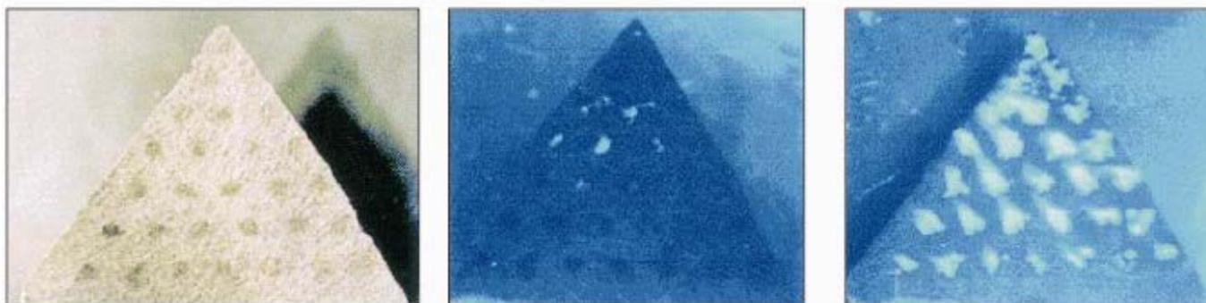
**Fig. 1.** Pt-Rh-Os ternary array in 6 M aqueous methanol (pH 6) quinine indicator. **(Left)** Image in white light. **(Center)** Fluorescence image at low overpotential, identifying the most active region of composition space. **(Right)** Fluorescence image at high overpotential, where methanol oxidation occurs at every spot in the array.
