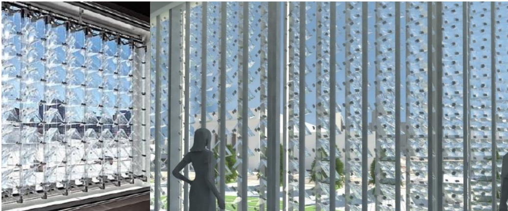
HeliOptix's Integrated Concentrating (IC) Solar Array: Solar heat and power collection that improves daylight resources, generates power, and controls solar gains.
