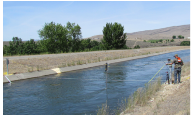
Figure 15. Sandia's mobile ADV deployment system for canal measurements. On top is the schematic of the system and a picture of the unit deployed in the field is shown on the bottom.
