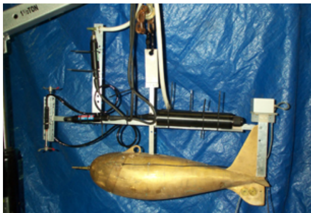
Figure 14. Cable-deployed ADVs (in circles) with sounding weight (Photograph courtesy of Bob Holmes, USGS, 2010).
