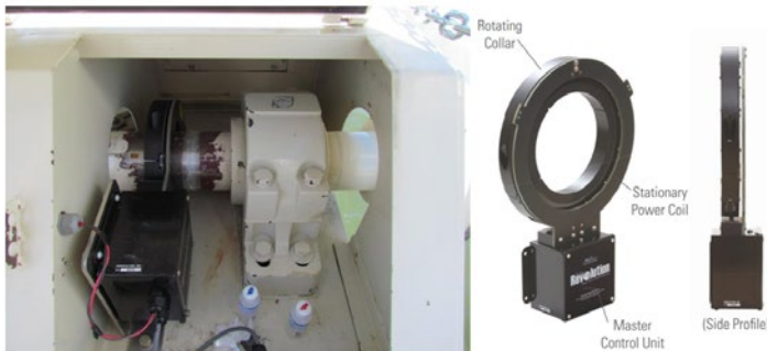
Figure 16. The torque sensor system mounted to the Instream’s turbine shaft at Roza Canal. The small brown rectangular sensor to the left of the torque sensor system is a strain gauge used for drag measurements.
