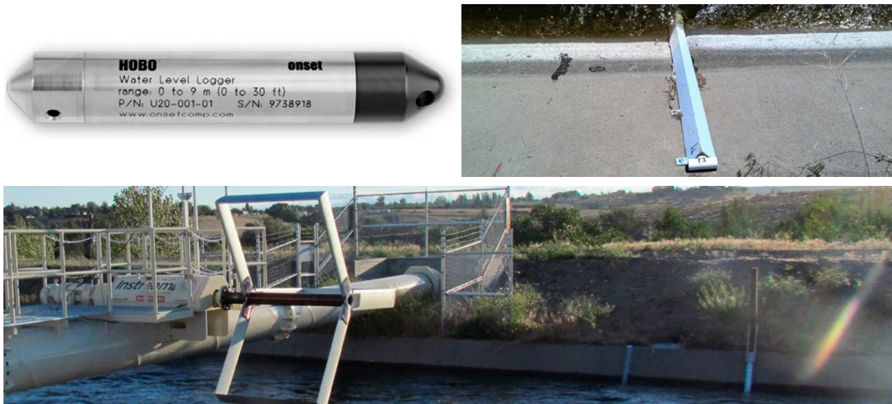
Figure 7. Top left: An example of water level pressure transducer; the length of the transducer in picture is 15 cm. Top right: Transducer, deployed using an angle iron anchored to the channel's side wall. Bottom: angle iron profiles mounted on the channel's side wall.
