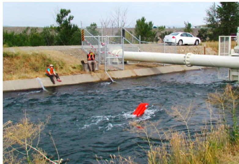
Figure 9. Boat capsize due to highly turbulent flow and uneven water surface downstream of a turbine.
