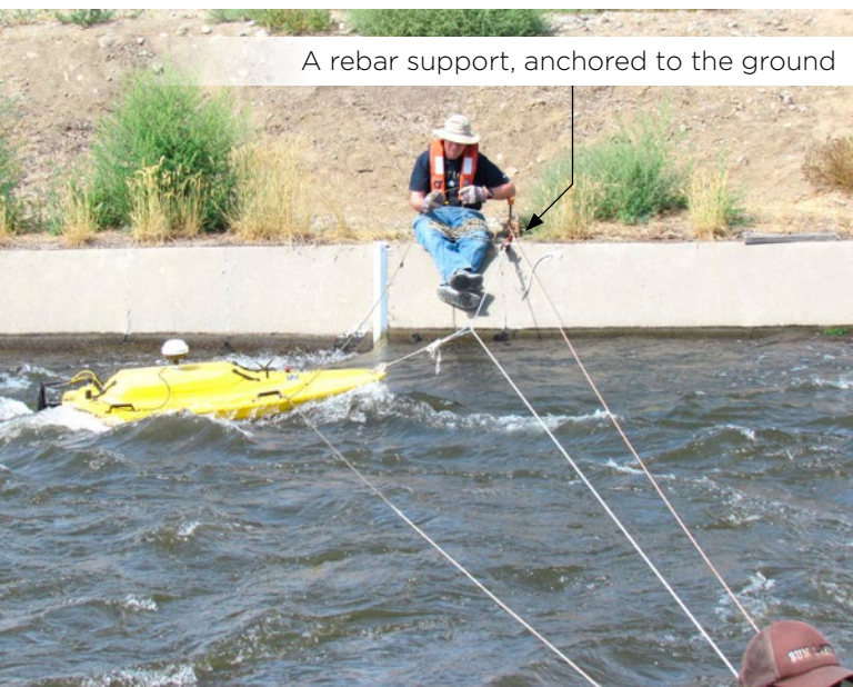
Figure 10. A cableway deployment with a tensioned tagline (the white line), that is attached to the ADCP boat.
