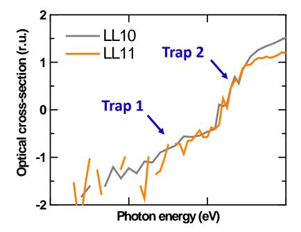
Energy levels of point defects are known from DLOS, but microscopic identities of the defects (impurity, atom vacancy, etc.) are not known
